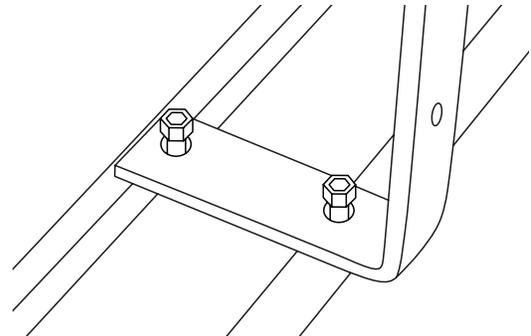
The shower awning can now be attached to the roof rack or roof bar as shown in the following diagrams. **IMPORTANT:** In some cases, 6.5mm holes will need to be drilled to attach brackets.
