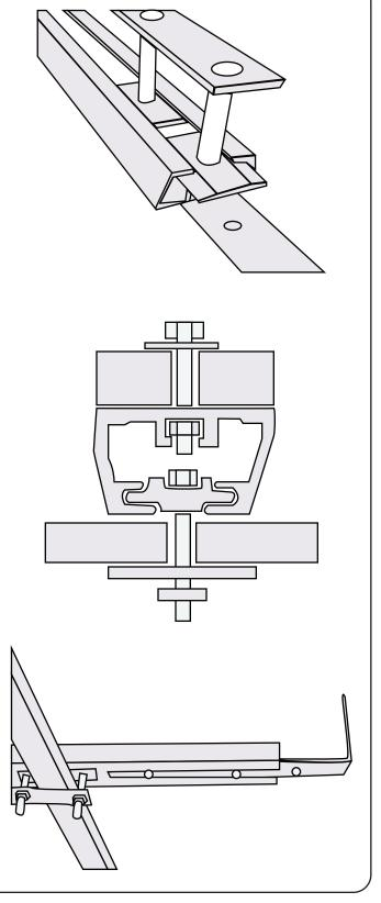
Align awning into desired position and tighten all nuts and bolts from previous steps.
