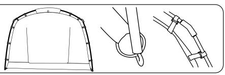
Insert the Long Pole through the holes in the center portion from the front to the rear of the tent.
