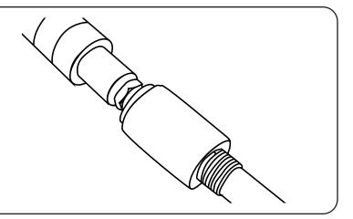
Determine the style of fitting on your compressor If it is a Nitto Fitting you will need to use our Nitto Adapter to connect the manifold
