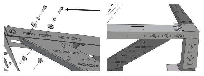
Select Side plate mounting bracket. Attach the mounting bracket to the bottom inside of the side plate with 8mm Torx bolts, 8mm Lock Washers, 8mm Flat Washers and 8mm Flange Nuts. Do not tighten hardware. Repeat this Step to attach the remaining Mounting Bracket to the Side Plate.
