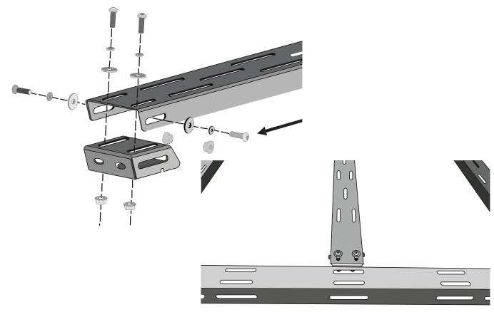
Locate the center slot in the Side rails. Attach the crossbar mounting brackets to the center slot in the side rails with 8mm Torx Bolts, 8mm Lock washers, 8mm Flat washers and 8mm Flat Nuts. Do not tighten hardware
