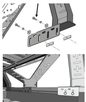
Level and adjust the Overland bed Rack and tighten all hardware.
