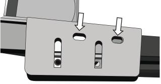
With a 5/16" Drill bit, (not included) drill through the bed. Replace the bed rack onto the bed.
