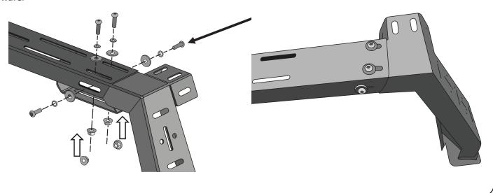
Select side rail and the Driver/Left rear support bracket. Attach the side rail to the front and rear support plates with 8mm Torx Bolts, 8mm Lock Washers, 8mm Flat Washers and 8mm Flange Nuts. Do not tighten hardware. Repeat this Step to attach the remaining side rail and the Passenger/Right support plate to the passenger/right side of the bed rack.
