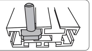
Place Mounting bracket onto the 2 T-Bolts as shown in Fig. 2
