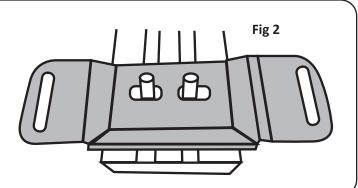
**Loosely Install washers and Nylock Nuts onto T-Bolts**
