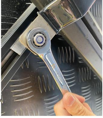
IMPORTANT: After installation, be sure to check all brackets to ensure everything is secure. Troubleshoot the tent by shaking the bushveld back and forth and possibly going for a short drive. Doing this will ensure that the tent doesn't shift.
