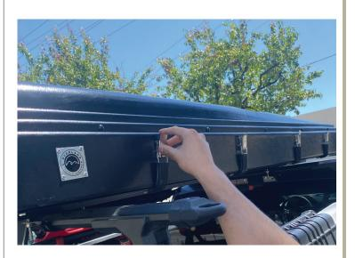
**2.**With your hand push up the hard shell handle. The gas struts will automatically open the rest of the tent on its own.
