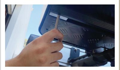
**3** Have a friend lift the Bushveld while a second person slides the piece over the crossbar so that one bolt is on each side of the bar.
