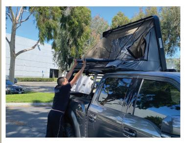
**4.** Grab the black nylon strap attached to the top of the shell (you may need the help of the rods of the canopy or climb to reach the strap). Pull down on the strap to close the hard shell.
