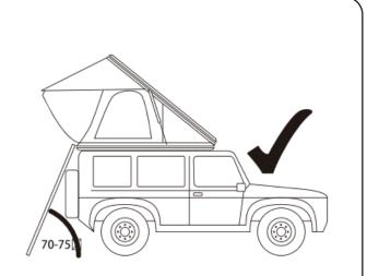
Once the tent is fixed securely to the vehicle's roof rack and the vehicle is positioned with the hand brake applied, attach the ladder, and ensure that it is secure and is locked in position and on an angle of 70 to 75 degrees.
