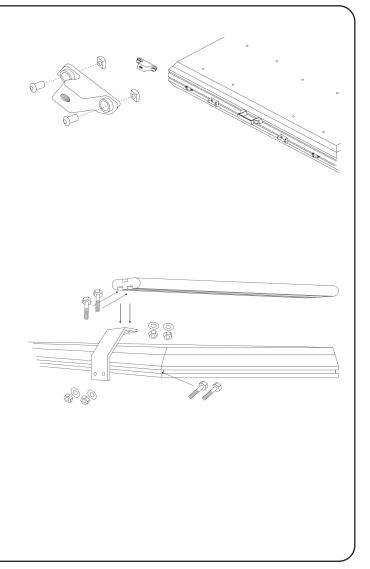
Place the tent on top of your vehicle rack system, ensuring the mounting tracks are perpendicular to the bars they will mount to, and the tent is centered on the roof rack.
