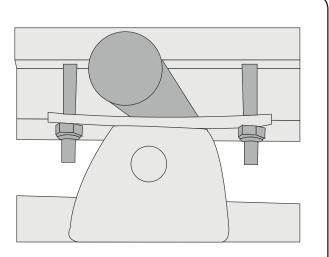
After ensuring the tent is positioned correctly and all eight bolts are tightened securely, insert rubber end caps into the ends of the mounting tracks. This may require light taps from a hammer.
