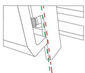
Note: Use a Torque Wrench (Ft-Lb) to tighten the clamping system down to your truck bed properly. You need at least 8-10ft-lbs of torque on the clamps to ensure they are secure to the bed. Any less and the cap may be in danger of moving or falling off when driving.
