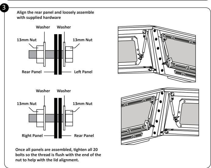
Notice for all customers, ANTI-SEIZE LUBRICANT MUST BE USED ON ALL STAINLESS STEEL FASTENERS TO PREVENT THREAD DAMAGE AND GALLING.
