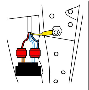
For the wiring to the 3rd brake light, Yellow Wire >White Wire Red Wire >Red Wire Blue Wire >Brown Wire
