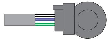
For the wiring to the 3rd brake light, Yellow Wire >White Wire Red Wire >Red Wire Blue Wire >Brown Wire
