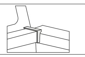
Set the Expedition Truck Cap on top of the vehicle. Take time to set evenly in place to eliminate damaging the 3M gasket.
