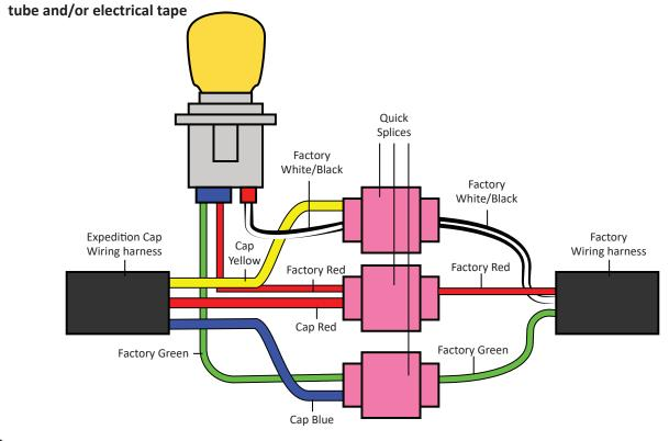
IT IS HIGHLY RECOMMENDED TO HAVE AUTOMOTIVE ELECTRONICS PROFESSIONAL COMPLETE THE INSTALLATION TO ENSURE THE THIRD BRAKE LIGHT FUNCTIONS CORRECTLY. TALK TO A WIRING SPECIALIST BEFORE SETTING UP THE WIRING PORTION.
