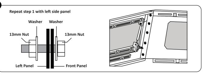
Align the rear panel and loosely assemble with supplied hardware
