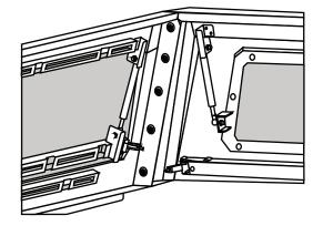
Once all panels are assembled, tighten all 20 bolts so the thread is flush with the end of the nut to help with the lid alignment.
