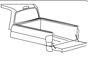
It is recommended to use the provided Butyl tape at the bulk head and bed rail seam.
