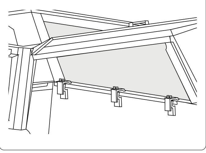
Alternate between the 2 13mm bolts to ensure that the clamp is providing even pressure and bolts do not strip.
