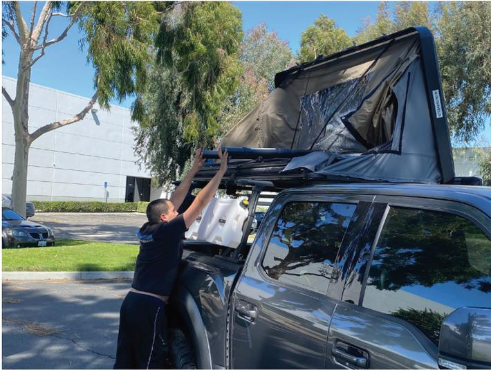
4. Grab the black nylon strap attached to the top of the shell (you may need the help of the rods of the canopy or climb to reach the strap). Pull down on the strap to close the hard shell.
