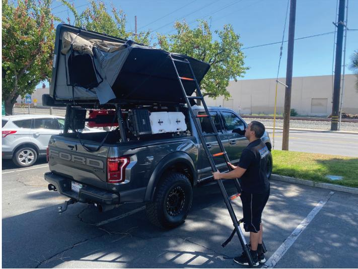
6. After the extended tent base has been lowered, secure the ladder by bringing the top rungs up from the top until they are locked into place one at a time.
