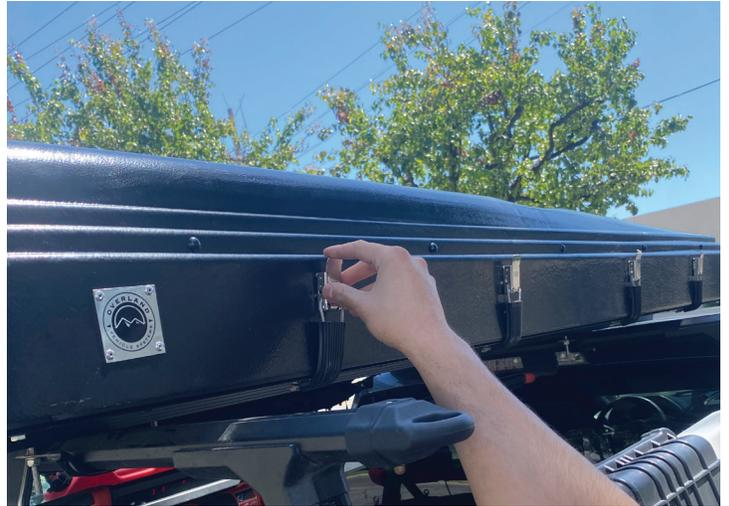
2. With your hand push up the hard shell handle. The gas struts will automatically open the rest of the tent on its own.
