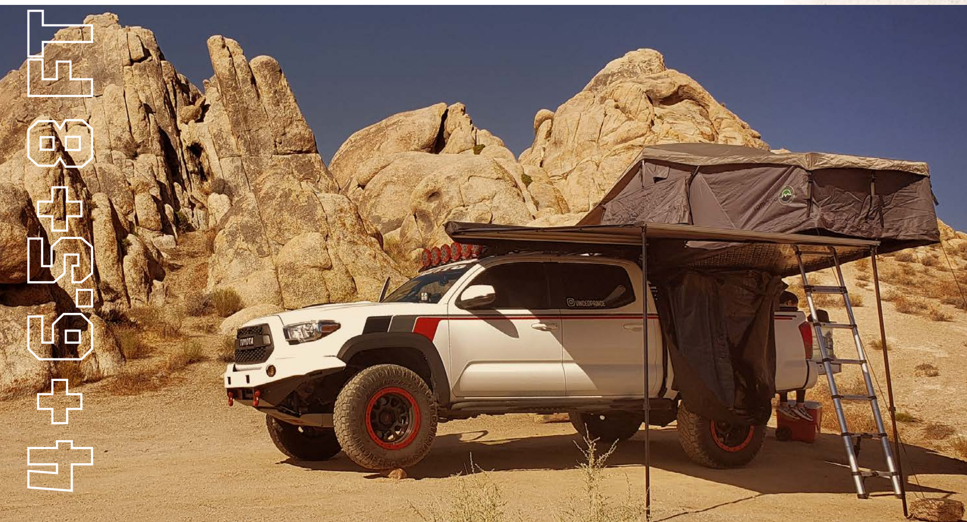
Pivoting aluminum support poles feature twist and lock technology adjustable up to 8.5 feet
