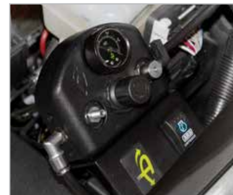
ADS Controller features 2 inlet valves for optional air sources.
