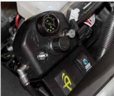
ADS Controller features 2 inlet valves for optional air sources.
