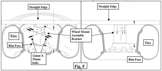
**Step 10:** Secure the tire mount bracket assembly (**outside**) and the 3rd brake light lower bracket (**inside**) to the tire carrier mount using the (**4**) supplied **12mmX 35mm** bolts and hardware. Torque **12mm** hardware to **80** ft./lbs. (Fig. G)
