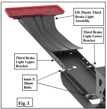
Step 14: Remove the (2) OE screws from the OE plastic third brake light assembly. Install the OE front plastic panel and lens into the new third brake light assembly using the (2) previously removed OE screws. (Fig. I)
