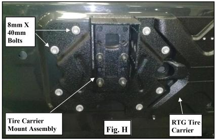
Step 12: Install the spare tire to the tire mount bracket and secure using the supplied lug nuts.
